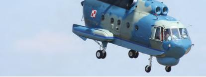
i-14 maritime helicopters in the PŁ (Anti-Submarine Warfare) version have been subject to not only a major overhaul, but also modernisation (test flight of the first upgraded helicopter No.1007 took place in 2001). This modernisation included fitting the aircraft with a modern radio and navigation suite, search and rescue (SAR) equipment as well as digital systems for both detection and engagement of submarines (dipped sonar, magnetic anomaly detector and sonobuoys).
